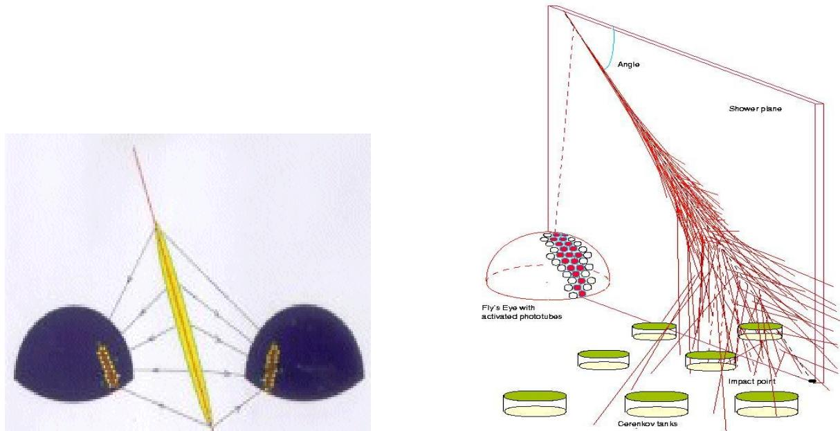
*Stereo Fluorescence or Hybrid Fluorescence + Ground Array precision measurements*
