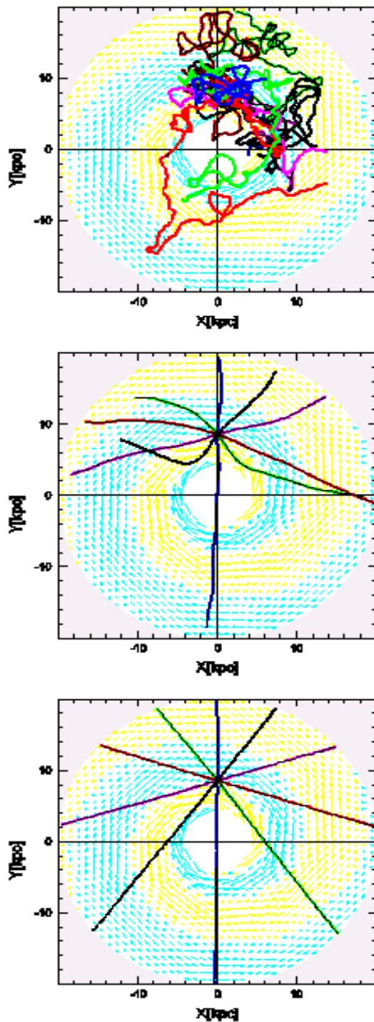
**Simulated proton trajectories:**  $10^{18}, 10^{19}$  and  $10^{20}$ eV in  $2\mu\text{G}$  fields ...  $\geq 4 \times 10^{19}$ eV protons are deviated little by local (galactic) magnetic fields.
