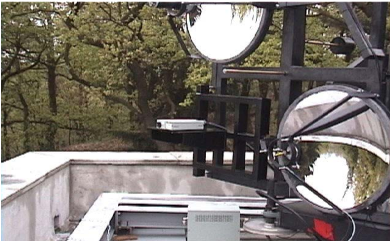
Prototype LIDAR testing at Pino Observatory near Torino.
