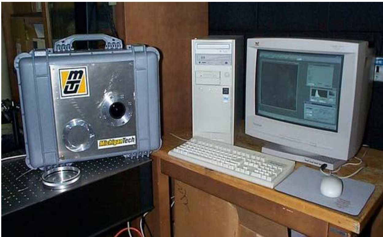
CONCAM photometer (in weather-proof enclosure) with control computer.
