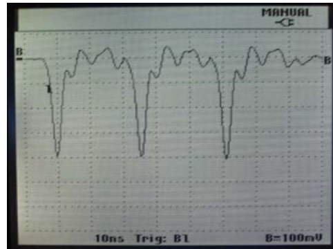
Fig. 4. The observed return-light time distribution from three separate calibration light paths. The 200 Mhz oscilloscope has somewhat limited bandwidth for the fast \sim 1 ns light pulses. The relative time delays between the three light paths is the result of the addition of 5m and 10m of (additional) optical fiber to two of the light paths. The near equality of the signals shows the good uniformity of the light coupling into the 1:37 output and 1:19 return optical fan-outs/fan-ins.
