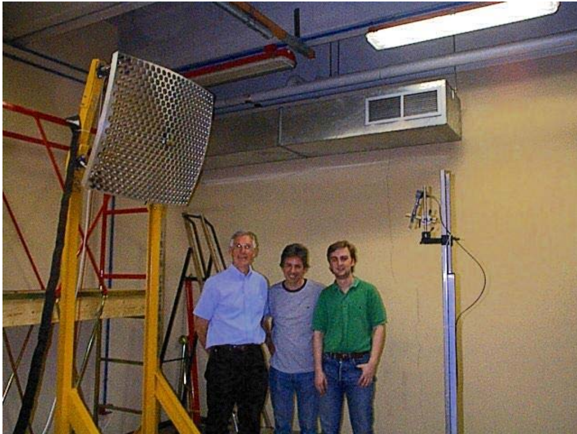
Fig. 2: Photograph of the University of Roma2 set-up: camera with three monitoring PMTs on the left and light source on the right. The light source was positioned at the nominal mirror center point.
