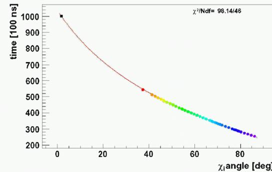
Adding SD timing to the FD reconstruction converts angular error *bananas* into *circles*
