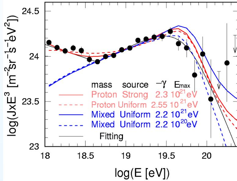
(Left plot) The Auger Flux  $\times E^3$  (ICRC'07). The suppression is “obvious” but quantification should be done carefully.
