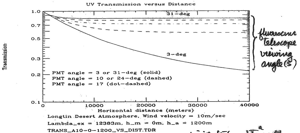
Fig. 2b: Transmission factor,  $T^a$  for Mie scattering on the aerosols in the atmosphere. The aerosols are described by a (horizontal) attenuation length  $\Lambda^a(350nm) = 12,383m$  and an exponential scale height,  $h_a = 1200m$  [3,4]. Curves are shown for HiRes viewing angles from  $3^\circ \sim 31^\circ$  to the horizon.
