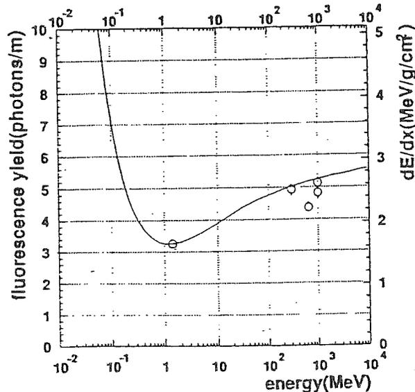
Fig. 7. Energy dependence of nitrogen fluorescence between 300 and 400 nm in dry air at a pressure of 760 mm Hg. The  $dE/dx$  curve is shown as a solid line. The scale of the fluorescence yield is adjusted so that the 1.4 MeV point lies on the  $dE/dx$  curve.
