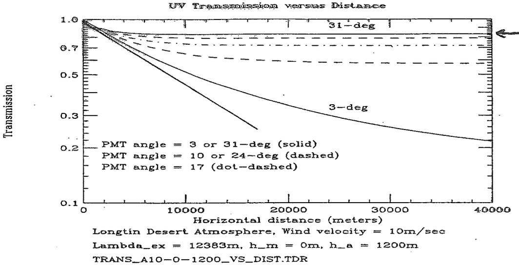
Fig. 3a': Transmission factor,  $T^a$ , for Mie scattering on the aerosols in the atmosphere. The aerosols are described by a (horizontal) attenuation length  $\Lambda^a(350nm) = 12,383m$  and an exponential scale height,  $h_a = 1200m$  [3,4]. Curves are shown for HiRes viewing angles from  $3^\circ \sim 31^\circ$  to the horizon.
