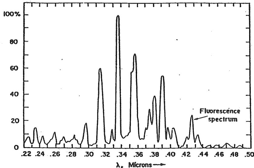
FIGURE 6.1 Spectrum of nitrogen fluorescence in the near ultraviolet.
