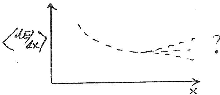
$$\langle \frac{dE}{dx} \rangle \equiv \frac{\Delta E \text{ available to air fluorescence}}{\Delta x N_e(x)}$$
